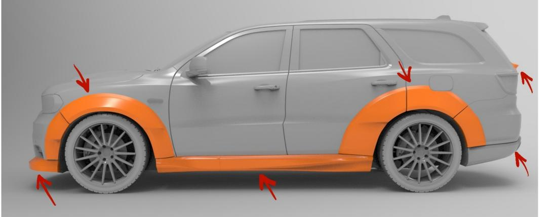
We are leaving some extra material on the edges in order for the installer to trim the edges to fit all body lines
